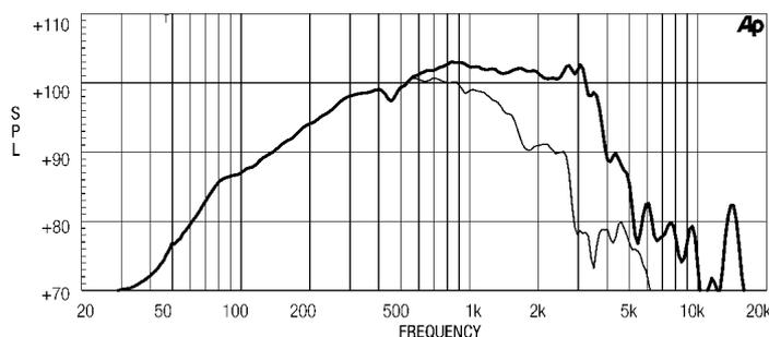
**FREQUENCY RESPONSE CURVE OF 12MB1000 MADE ON 50 LIT. CLOSED BOX ENCLOSURE IN FREE FIELD (4PI) ENVIRONMENT. ENCLOSURE CLOSES THE REAR OF THE DRIVER. THE THIN LINE REPRESENTS 45 DEG. OFF AXIS FREQUENCY RESPONSE**
