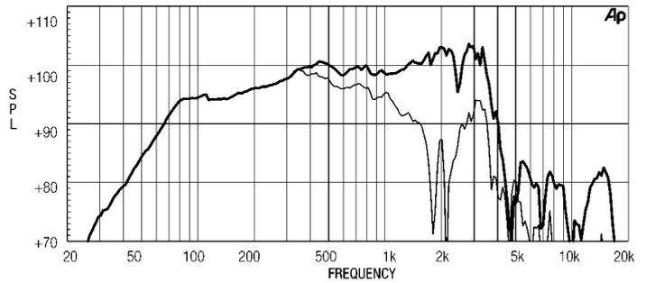
**FREQUENCY RESPONSE CURVE OF 15MB1000 MADE ON 125 LIT. ENCLOSURE TUNED 50HZ IN FREE FIELD (4PI) ENVIRONMENT. ENCLOSURE CLOSES THE REAR OF THE DRIVER. THE THIN LINE REPRESENTS 45 DEG. OFF AXIS FREQUENCY RESPONSE**
