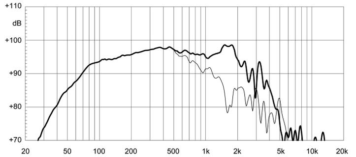
**FREQUENCY RESPONSE CURVE OF 15NLW9300 MADE ON 125 LIT. ENCLOSURE TUNED AT 50HZ IN FREE FIELD (4PI) ENVIRONMENT. ENCLOSURE CLOSES THE REAR OF THE DRIVER. THE THIN LINE REPRESENTS 45 DEG. OFF AXIS FREQUENCY RESPONSE.**
