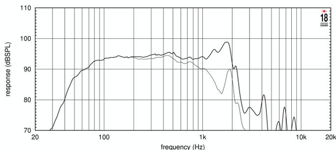
**FREQUENCY RESPONSE CURVE OF 15NLW9401 MADE ON 125 LT. ENCLOSURE TUNED AT 50HZ IN FREE FIELD (4PI) ENVIRONMENT. ENCLOSURE CLOSES THE REAR OF THE DRIVER. THE THIN LINE REPRESENTS 45 DEG. OFF AXIS FREQUENCY RESPONSE.**
