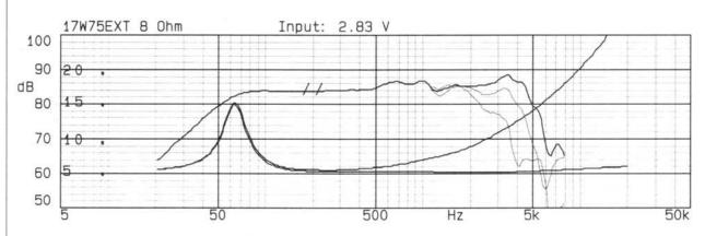
Frequency response 17 W-75 EXT on-axis, 30° and 60°, distance 1m, 8 ohm version. Impedance curve with and without correction circuit (6.8 ohm and 20  $\mu$ F).
