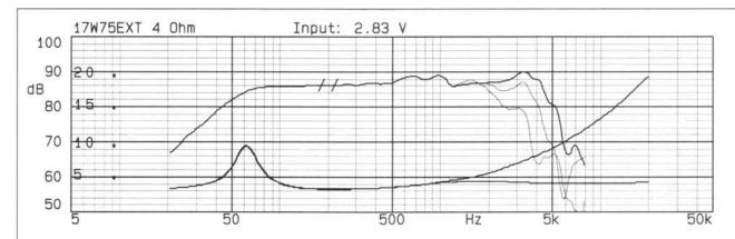
Frequency response 17 W-75 EXT on-axis, 30° and 60°, distance 1m, 4 ohm version. Impedance curve with and without correction circuit (4.7 ohm and 15  $\mu$ F).
