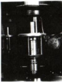
Combining different materials together requires experience and know how about the behavior even under extrem conditions. - Here we glue aluminum former to the fabric spider. An exact amount of high temperature resistant glue is precisely placed to the spiders neck. The voice coil of the woofer survives temperature peaks of even 400 to 650°F (300-400°C). Furthermore the connection point has to withstand accelerations of some hundred miles/h altering the direction some thousand times per second.
