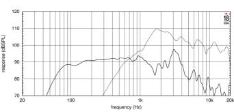
FREQUENCY RESPONSE MADE IN 25 LT. ENCLOSURE TUNED AT 65 Hz IN FREE FIELD (4n) ENVIRONMENT. ENCLOSURE CLOSES THE REAR OF THE DRIVER, THE THIN LINE REPRESENTS HIGH FREQUENCY
