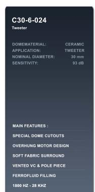
The C30 - 6 - 024 is a 1.2 inch tweeter with ultra hard ceramic dome in a 82 mm frontplate.
