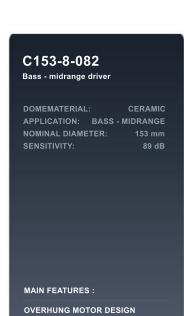
The C153 - 8 - 082 is a 5 inch bass - midrange driver with ultra hard ceramic dome.
