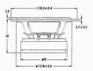
The W14CY-001 is a 5" cone driver developed for use as a high fidelity Woofer or Woofer/Midrange unit. The extremely stiff, yet light cone gives tremendous bass precision and midrange detail.
