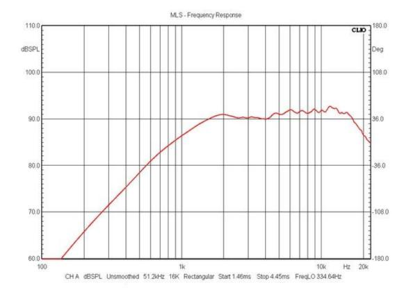
Frequency response from a more appropriate off-axis mounting on a 200 mm front panel with 7, 8 and 12 cm to nearest edges.
