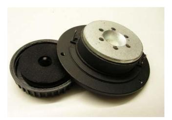
Six holes in magnet poleplate provide proper ventilation of voice coil, ensuring minimum compression and voice coil cooling.
