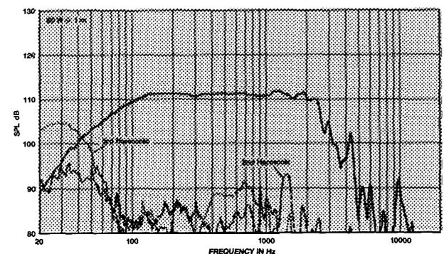
Distortion levels raised 20 dB, measured at 60 watts, 1 meter.
