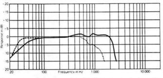
Frequency response contour of the 2245H taken in a hemispherical free-field environment, a closed box of 280 L (10 ft\*) internal volume enclosing the rear of the driver. Measured response of a typical production unit, including all peaks and dips, does not deviate more than 2 dB from the above curve. The dashed curve represents the response from a 320 cm² (50 in²) port with a 20 cm (8 in) long duct tuning this enclosure to 30 Hz.
