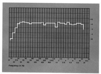
Frequency response of the 4345 taken with 1/3-octave band pink noise. Measured response contour of a typical system averaged through an inclusive arc of 60° in the horizontal and 30° in the vertical planes does not deviate more than 2 dB from the above curve.
