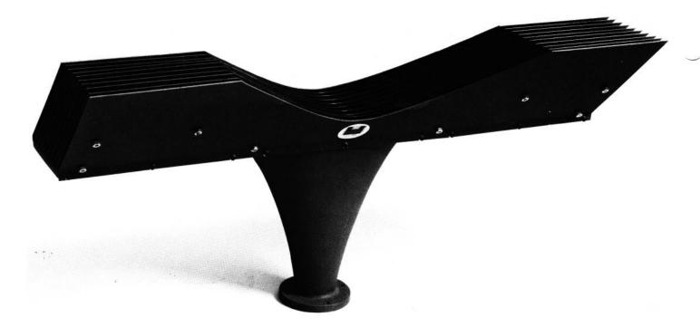
The JBL 2395 is a slant-plate acoustic lens for use above 800 Hz. Sensitivity 108 dB. The horizontal pattern of 140° is determined by the shape of the plates. The lens is backed up by a 300 mm (12 in) elliptical exponential horn. The 45° vertical pattern is closely controlled by the shape of this horn. The lens does not require additional baffling for use above 800 Hz. To insure proper high frequency operation the ends
