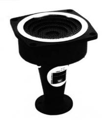
The JBL 2301 is a perforated plate acoustic lens for use above 1200 Hz. It is intended for use as the high frequency element in a two or three frequency band integrated system where the length of throw does not exceed 9 m (30ft). Above 1200 Hz, the pattern has a conical shape with an included angle of 90.° Sensitivity 109 dB. The 2301 will accept 25 mm (1 in) drivers only. Nominal Q=4 (2 kHz octave band).
