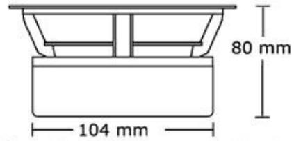
fixing holes 4 x 5mm on 132 PCD
