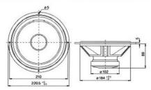
High-End CC line 8" woofer with low resonance. This woofer has got all the good features of the CC line programme such as short circuiting ring and spacer. It has rubber surround and an extra thick polypropylene cone. The low resonance makes it ideal for use as subwoofer and it is also very suitable for closed and reflex boxes two or three-way.
