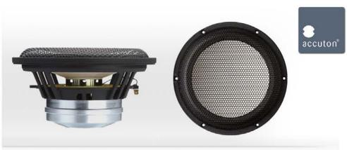
MAIN FEATURES : UNDERHUNG MOTOR DESIGN 55 MM TITANIUM VC FORMER SOFT RUBBER SURROUND VENTED VC, POLE PIECE & SPIDER 31 HZ - 1 KHZ IN VENTED BOX
