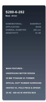
The **S280 - 6 - 282** is an 10 inch bass driver with ultra hard ceramic - sandwich dome.
