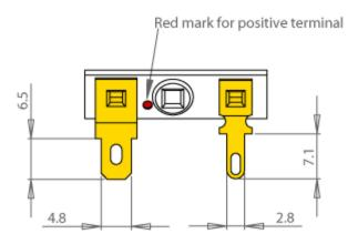
Thickness, both terminals: 0.5mm Terminal plating: Gold
