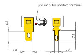
Thickness, both terminals: 0.5mm Terminal plating: Gold
