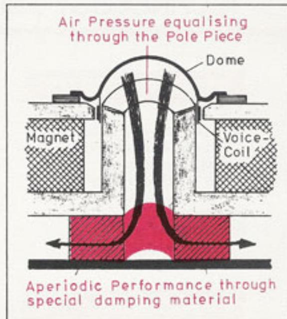
The advantages of the aperiodic damping are consequently applied to all DYNAUDIO dome constructions and may be achieved to all cabinet enclosures by using the VARIOVENT. Aperiodic damping may be compared with a shock absorber in a motor car. Physically the aperiodic damping acts like a DC-resistance in the oscillating circuit.
