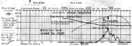
Exceptional linear phase response up to 40 kHz. The h.d. is measured at 110 dB.SPL!
