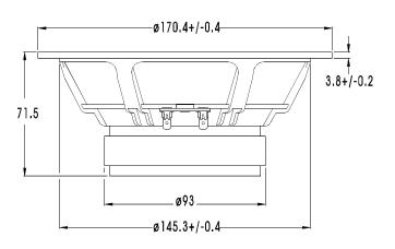
The W17E-001 is a 6,5" cone driver for use as a high fidelity Woofer or Woofer/Midrange unit. Choose it when you want smooth extended frequency response, linearized driving force, and low distortion.
