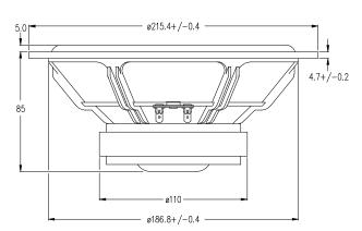
The W21EX002 is an 8" cone driver developed for use as a high fidelity Woofer or Woofer/Midrange unit. The extremely stiff, yet light cone gives tremendous bass precision and midrange detail.
