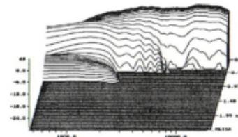
The MLSSA cumulative spectral decay (waterfall) plot shows the energy/time response of the ESOTEC® D-260. These fairly outstanding results clearly show that time delayed reflections have been reduced to a minimum.
