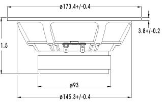
P17RCY is a 6,5" High Fidelity woofer with an injection moulded metal chassis, intended for bass reflex and transmission line designs. A specially compounded poly-propylene cone, a soft PVC dust cap and a high loss rubber surround yield a smooth and uncoloured response and high consistency. A high temperature voice coil wound on an aluminium voice coil former gives a high power handling capacity. The large magnet system provides high efficiency and low Q.
