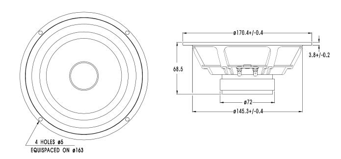
P17RC is a 6,5" High Fidelity woofer with an injection moulded metal chassis, intended mainly for closed cabinet designs. A specially compounded polypropylene cone, a soft PVC dust cap and a high loss rubber surround yield a smooth and uncoloured response and high consistency. A high temperature voice coil wound on an aluminium voice coil former gives a high power handling capacity.
