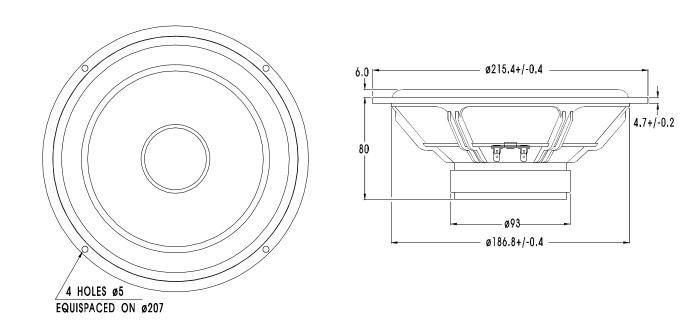
CA21RE is an 8" High Fidelity woofer with an injection moulded metal chassis. This unit has excellent mechanical matching between a paper cone, a paper dust cap and a low loss rubber surround. A special treatment of the cone produces a well behaved roll off characteristic and reduces potential resonance problems. The magnet system has a T-shaped cross section of the pole piece for low modulation distortion. A relatively large voice coil diameter gives a high power handling capacity.
