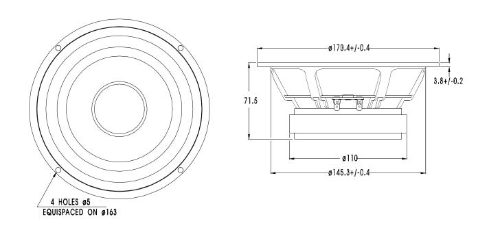
P17REX is a 6,5" High Fidelity woofer with an injection moulded metal chassis. A polypropylene based cone, a soft PVC dust cap and a high loss rubber surround are carefully matched to each other, resulting in an outstandingly smooth frequency response. The unit has a high power handling capacity due to its relatively large voice coil diameter. The magnet system has a T-shaped cross section of the pole piece for low modulation distortion. A large magnet system provides high efficiency and low Q.
