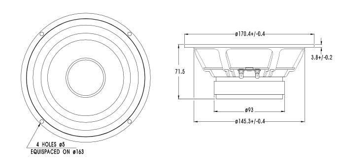
T17RE is a 6,5" High Fidelity woofer with an injection moulded metal chassis. A PP/TPX based cone, a soft PVC dust cap and a high loss rubber surround are carefully matched to each other, resulting in an outstandingly smooth frequency response. The unit has a high power handling capacity due to its relatively large voice coil diameter. The magnet system has a T-shaped cross section of the pole piece for low modulation distortion.
